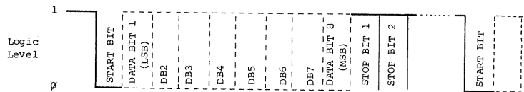
FIGURE 2-8a Typical asynchronous-serial bit pattern for the transmission of an 8-bit data word with 2 stop bits.
